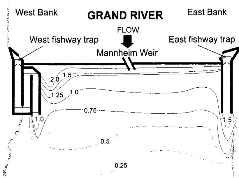
FIGURE 2.—Schematic of the fishways (not to scale) and the region immediately downstream from the Mannheim weir. Shaded areas in the fishways indicate the reception zones monitored by the underwater telemetry antennas. Relative velocity isopleths indicate surface water velocities (m/s) downstream from the weir, as measured with a Sigma PVM velocity meter.
